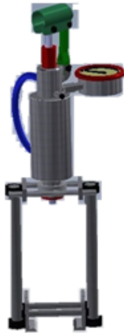
Figure 2. Desain Tracker Hidrolik Pelepas bearing kruk as (outer bearing).
