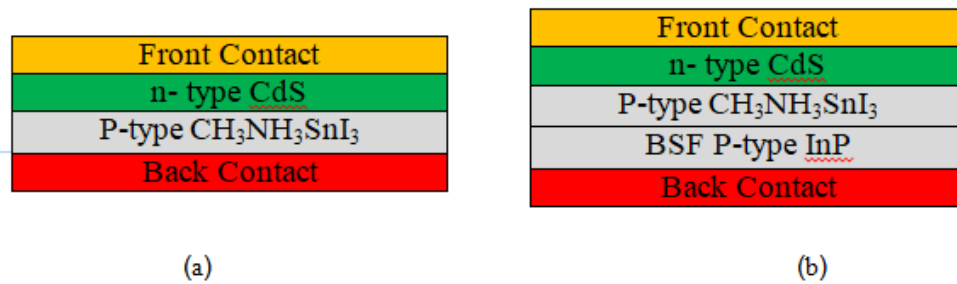
Figure 1. Perovskite solar cell (1) without and (2) with BSF layer (a) device structure and (b) energy payoff
