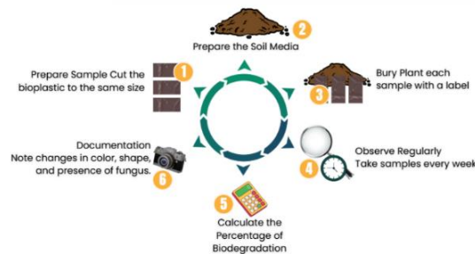
Figure 5. Schematic Illustration of the Soil Burial Biodegradation Test Procedure for PLA-Banana Peel Bioplastic
