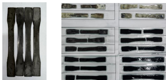
Figure 6. Tensile Test Specimen Shape of PLA and Banana Peel Flour Bioplastic
