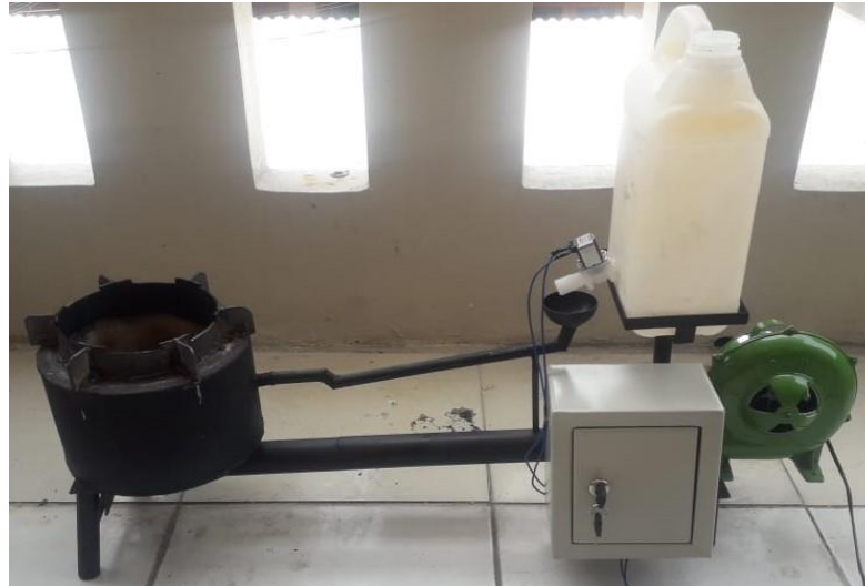
Figure 4. Prototype 2 Stove Fueled by Waste Cooking Oil with Automatic Fuel Supply System
