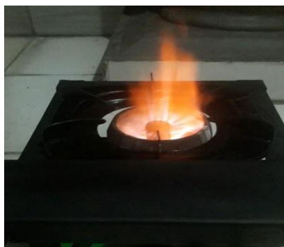
Figure 1. Prototype-1 Stove Using Used Cooking Oil as Fuel In The First Research
