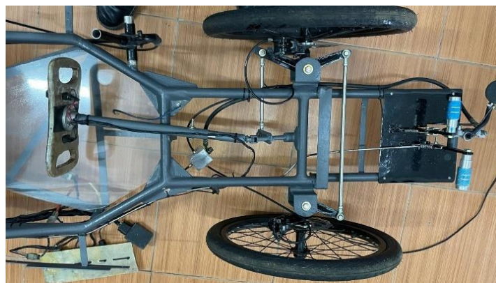
Figure 1. Integration of the fabricated steering subsystem during the manufacturing process. The steering column with universal joint, intermediate shaft, center bracket, and left/right tie-rods are mounted with M8 fasteners; clearances and wheel centering were verified before static tests.
