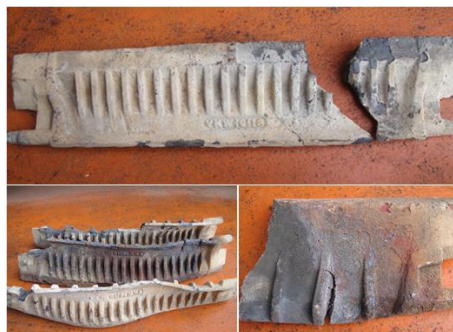
Figure 2. Failed grade bar
