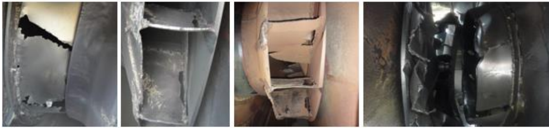
Figure 1. Faulty IDF fan blade and cone
