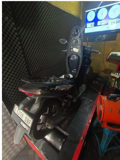
Figure 1. Beat Deluxe motorbike process on the dynotest machine
