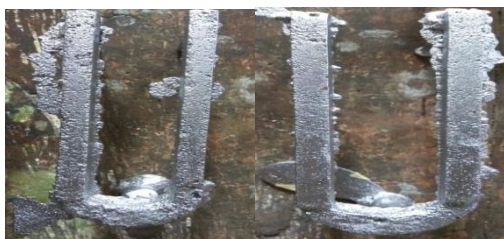
(a) Tanpa Holding time (b) Holding time 10 menit
